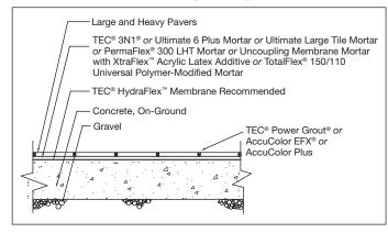
Interior Floors over On-Ground or Above Ground Concrete (TCNA F113)
