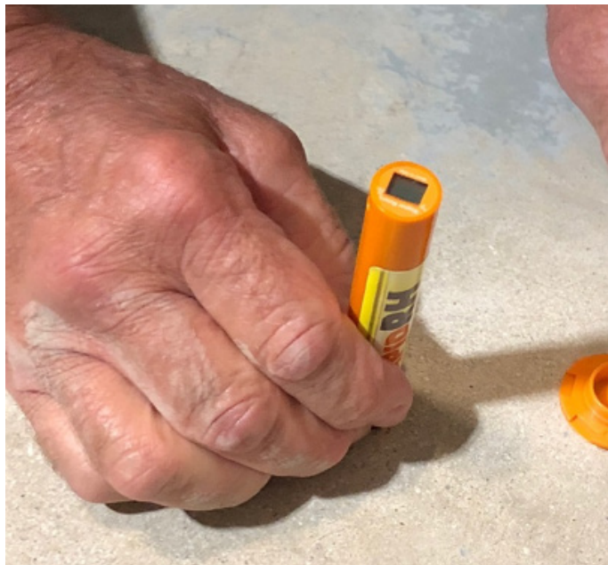
Figure 1. Probe being used to check relative humidity within slab according to ASTM F2170
