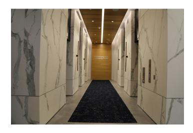
Throughout the project, **TEC** Power Grout was used for its ability to choose a color that was a great match to the actual porcelain. In areas with transitions, TEC AccuColor Premium Sanded Grout was chosen for its elasticity to avoid breakage with metal and porcelain. It created a good seal.
