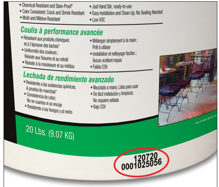
Figure 2. Example of an SAP batch number for liquid products showing this product was made on December 7 th , 2020.
