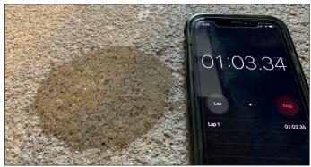
Figure 1. Water droplet partially absorbed after 1 minute indicating concrete is porous
