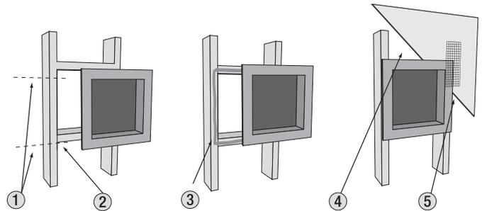
1. Position niche and mark the top and bottom of the flange between two studs (located 16" on center).
