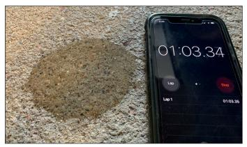
Figure 1. Water droplet partially absorbed after 1 minute indicating concrete is porous
