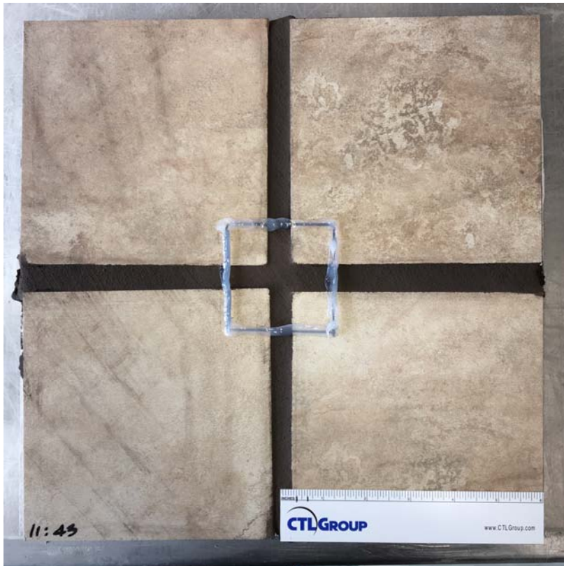
Figure C-1. Hydroment® Vivid™ - Bostik in Flash Walnut grout sample at 28 days of curing before efflorescence emittance test
