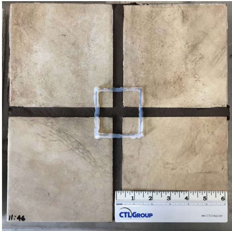
Figure B-1. Hydroment® Vivid™ - Bostik in Flash Walnut grout sample at 7 days of curing before efflorescence emittance test
