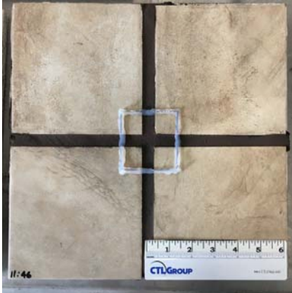
Figure 1. Grout sample tile with silicone caulk dam around center
