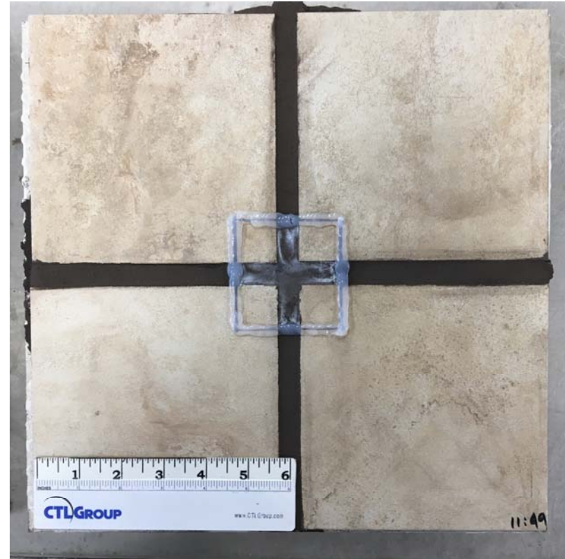
Figure A-2. Hydroment® Vivid™ - Bostik in Flash Walnut grout sample at 3 days of curing after efflorescence emittance test
