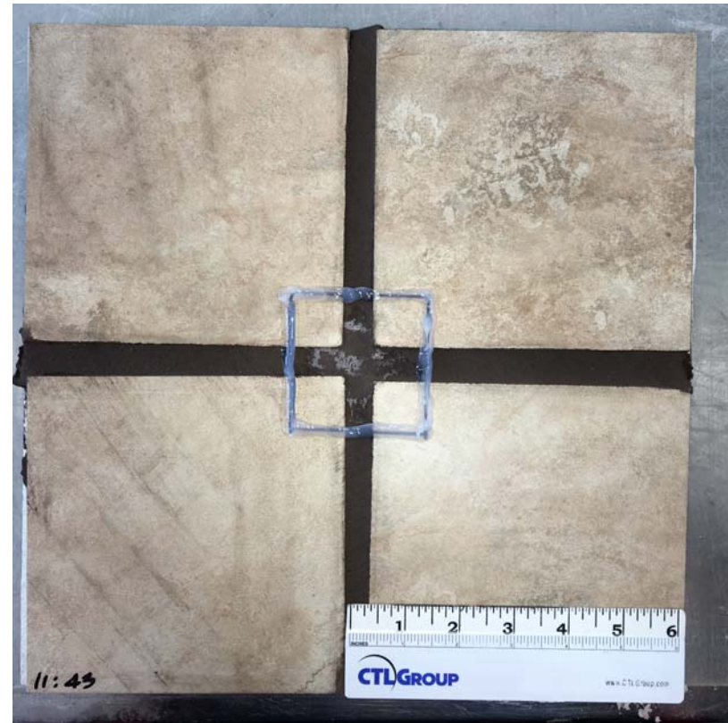
Figure C-2. Hydroment® Vivid™ - Bostik in Flash Walnut grout sample at 28 days of curing after efflorescence emittance test
