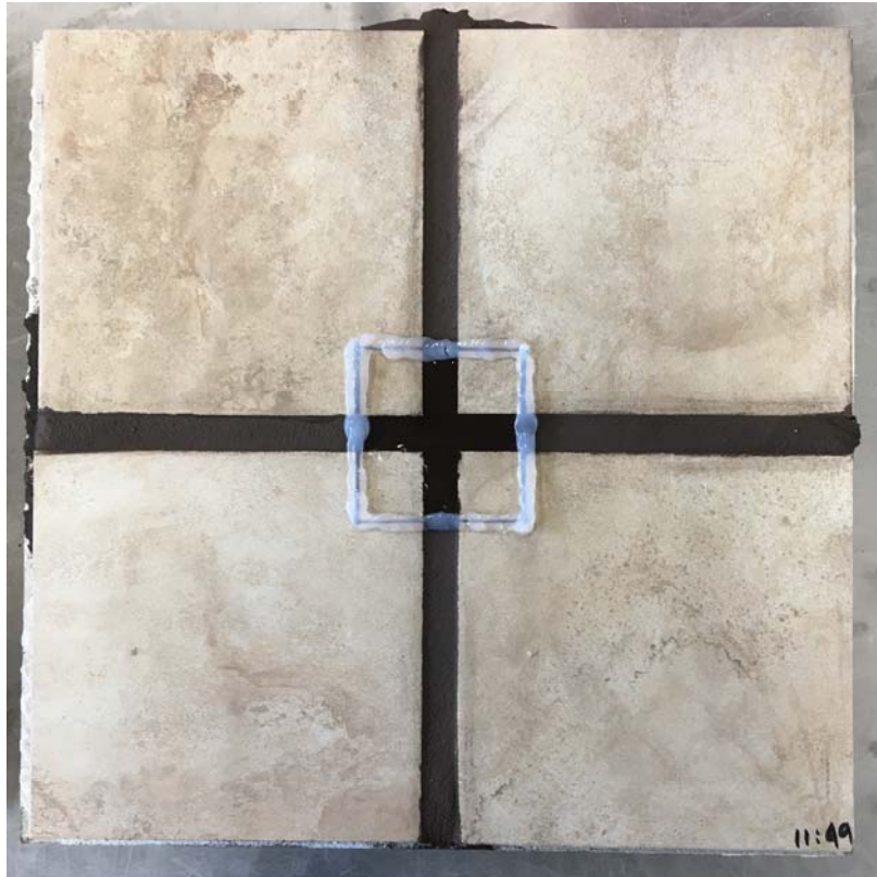
Figure A-1. Hydroment® Vivid™ - Bostik in Flash Walnut grout sample at 3 days of curing during efflorescence emittance test
