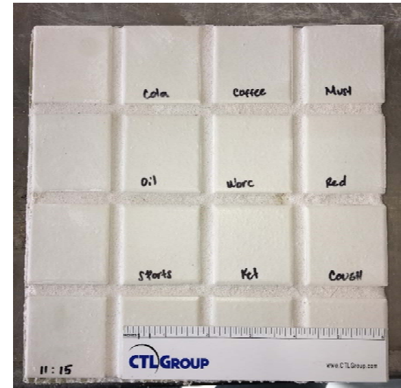
Figure 3. Specimen 1 of Hydroment® Vivid™ - Bostik (Bright White) after washing
