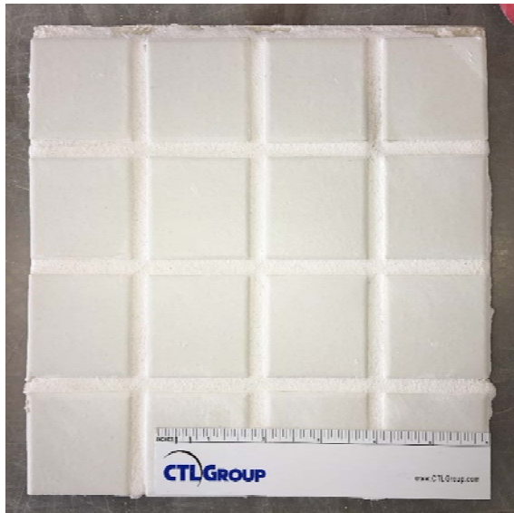
Figure 4. Specimen 2 of Hydroment® Vivid™ - Bostik (Bright White) before stain application
