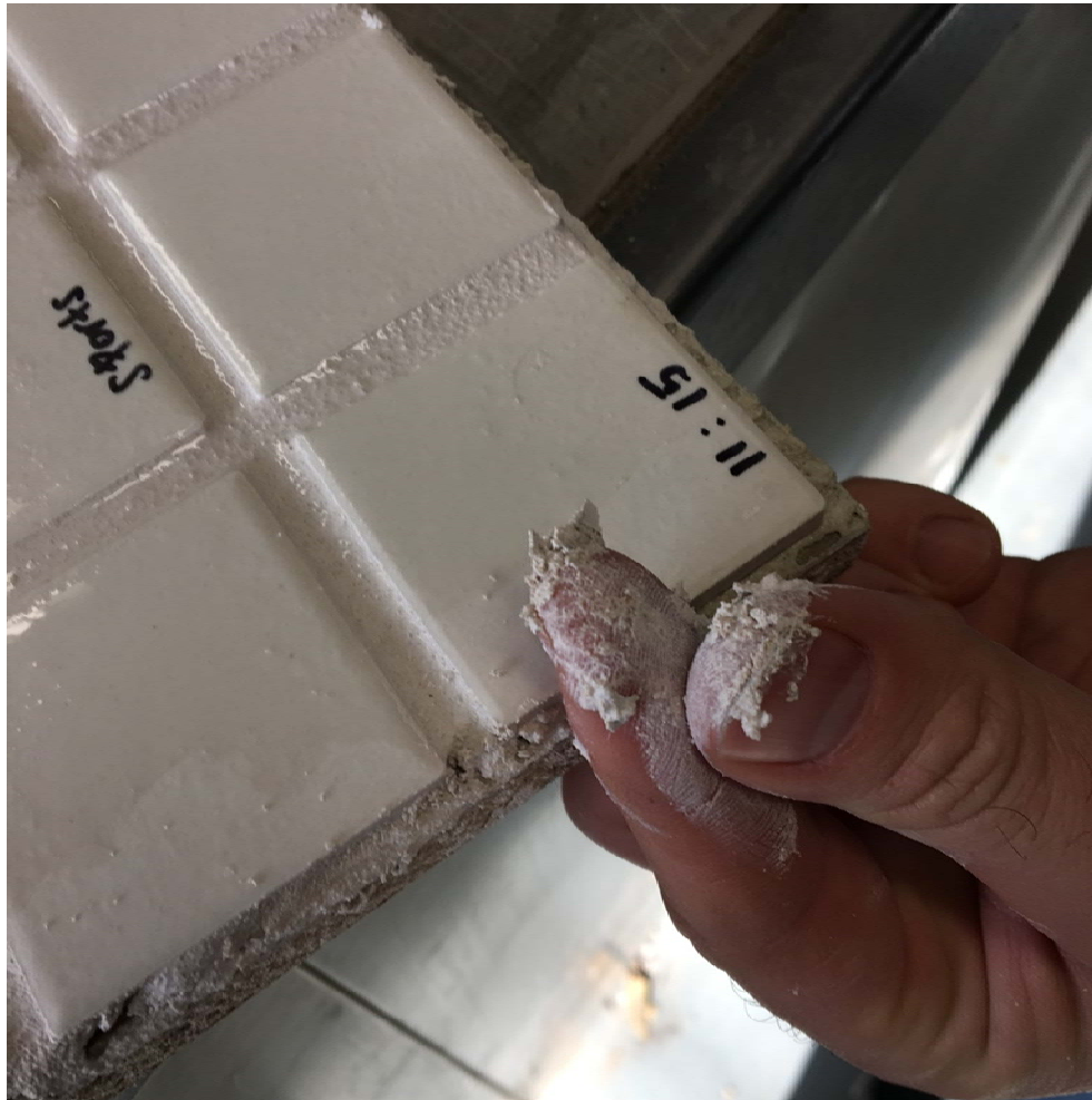
Figure 7 Detail of softened grout product after washing with water.
