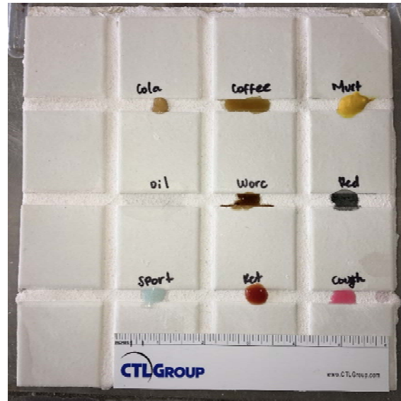
Figure 5. Specimen 2 of Hydroment® Vivid™ - Bostik (Bright White) during stain application
