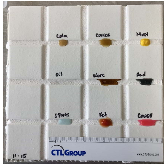
Figure 2. Specimen 1 of Hydroment® Vivid™ - Bostik (Bright White) during stain application
