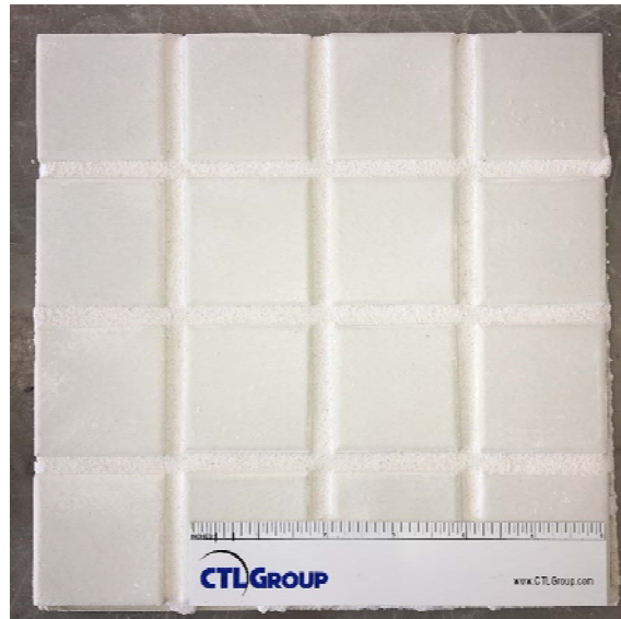
Figure 1. Specimen 1 of Hydroment® Vivid™ - Bostik (Bright White) before stain application
